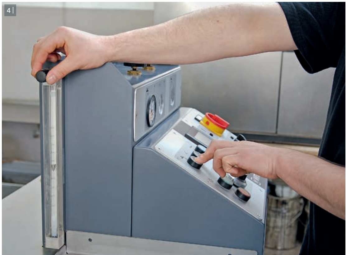
4 | Precise process water settings enable determination of the ideal foamed bitumen quality.
